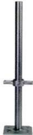
Adjustable Base or Screw Jack 32/34/36/38 mm (OD) 450/550/650/750 mm (Length) 100/150 mm (Safety Lock) Solid or Hollow Self Finish / Electroplated
