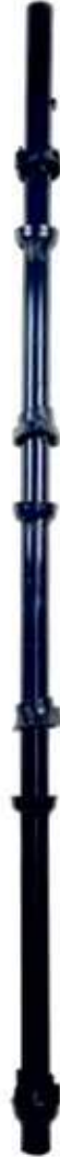
Standard Made from tube of 48.3 mm OD Available thickness (in mm): 3.0, 3.2, 4.0 Available Sizes (in mtr): 0.5, 1.0, 1.5, 2.0, 2.5, 3.0
